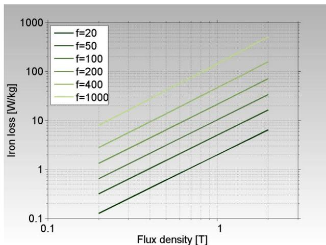
**Figure 4: Iron loss as a function of flux density at different frequencies - at a mechanical density of 7.57 g/cm<sup>3</sup>.**
