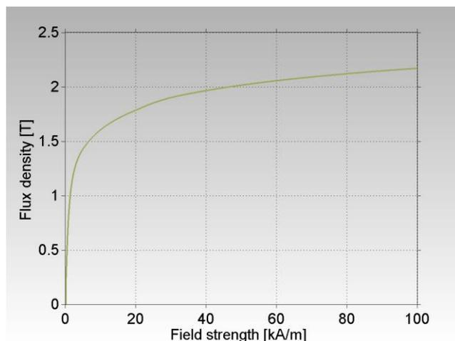
Figure 1: B-H curve for STX S7 SMC - at a mechanical density of 7.57 g/cm<sup>3</sup>.
