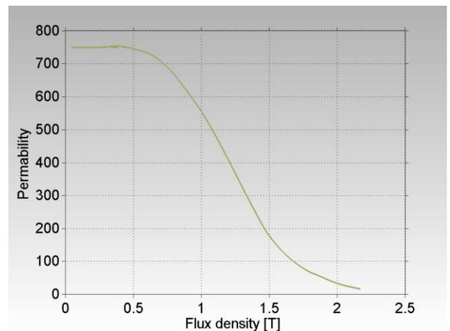
Figure 2: Permeability as a function of flux density for STX S7 SMC - at a mechanical density of 7.57 g/cm<sup>3</sup>.
