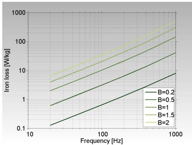
**Figure 3: Iron loss as a function of frequency at different flux densities - at a mechanical density of 7.57 g/cm<sup>3</sup>.**
