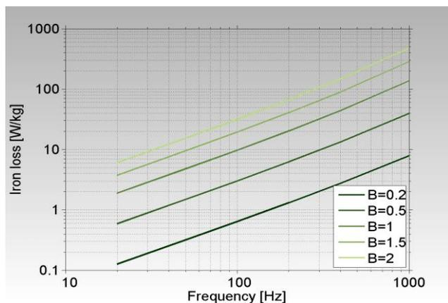
Figure 3: Iron loss as a function of frequency at different flux densities - at a mechanical density of 7.45 g/m³.
