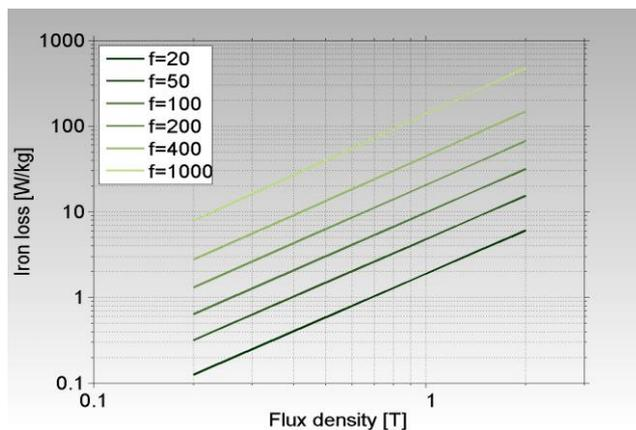
Figure 4: Iron loss as a function of flux density at different frequencies - at a mechanical density of 7.45 g/m³.
