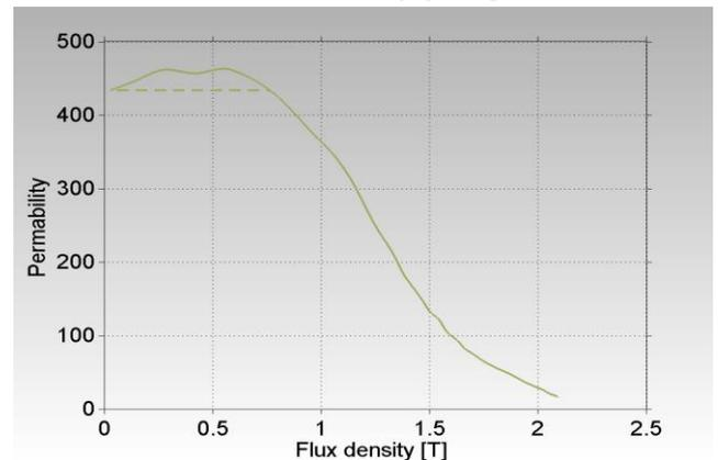
Figure 2: Permeability as a function of flux density for STX SMC material - at a mechanical density of 7.45 g/m<sup>3</sup>.
