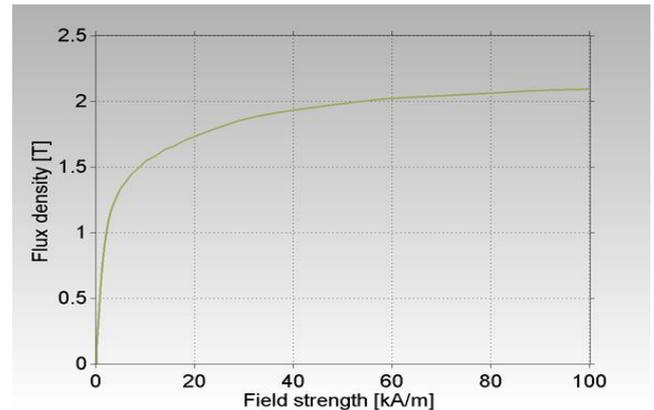
Figure 1: B-H curve for STX SMC Prototyping material - at a mechanical density of 7.45 g/m<sup>3</sup>.
